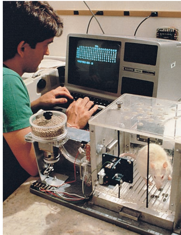
Figure 7.6 Apparatus for Instrumental Conditioning: the Operant Chamber. This photograph shows an operant chamber (often called a 'Skinner box') with a magazine for delivering food pellets. The computer is used to control the experiment and record the rat's responses.
